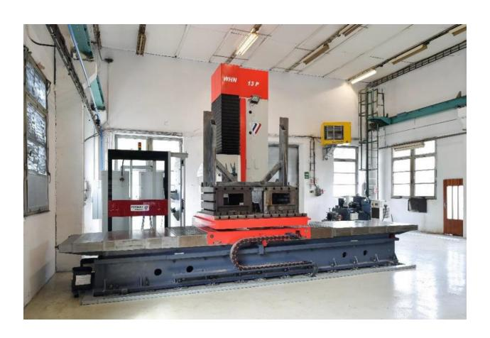
X / Y / Z / W (axes travels) 3 500 / 2 000 / 1 250 / 800 mm 137.7" / 78.7" / 49.2" / 31.4"
